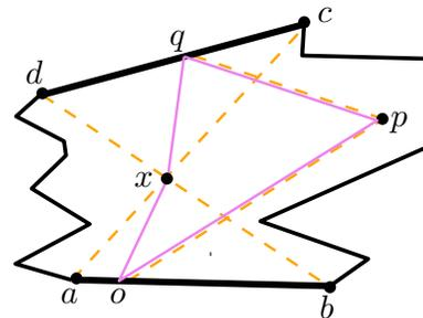
Figure 4: A schematic of the proof that a simple polygon with two open guard edges must be starshaped. The guard edges are  $ab$  and  $cd$ . The point  $x = ac \cap bd$  is in the kernel of the polygon, since every point  $p \in P$  is visible from  $x$ .
